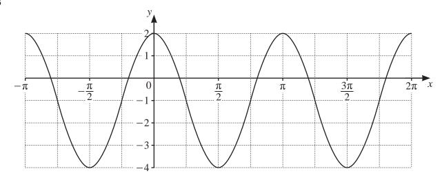
(a) The curve has equation  $y = a \cos bx + c$  where a, b and c are integers. Find the values of a, b and c. [3]
